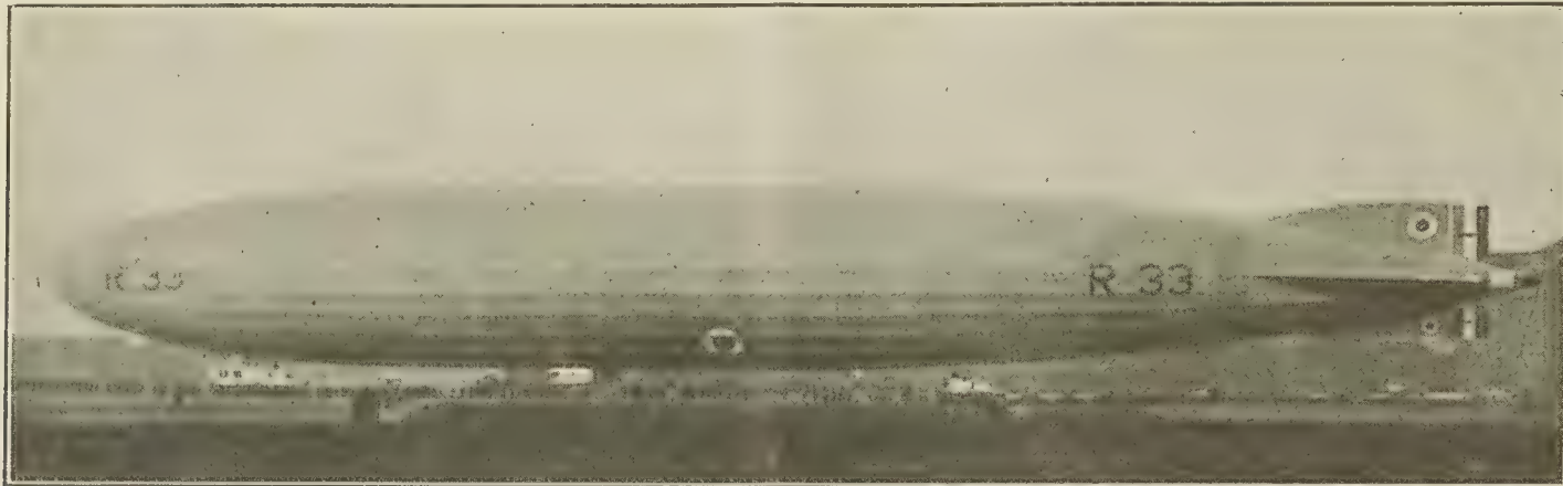
British Rigid Airship, R 33; Hp., 1250; speed, 70 m.p.h.; length, 670 ft.; master diameter, 79 ft.; disposable lift, 29 tons Photo International Film Service
